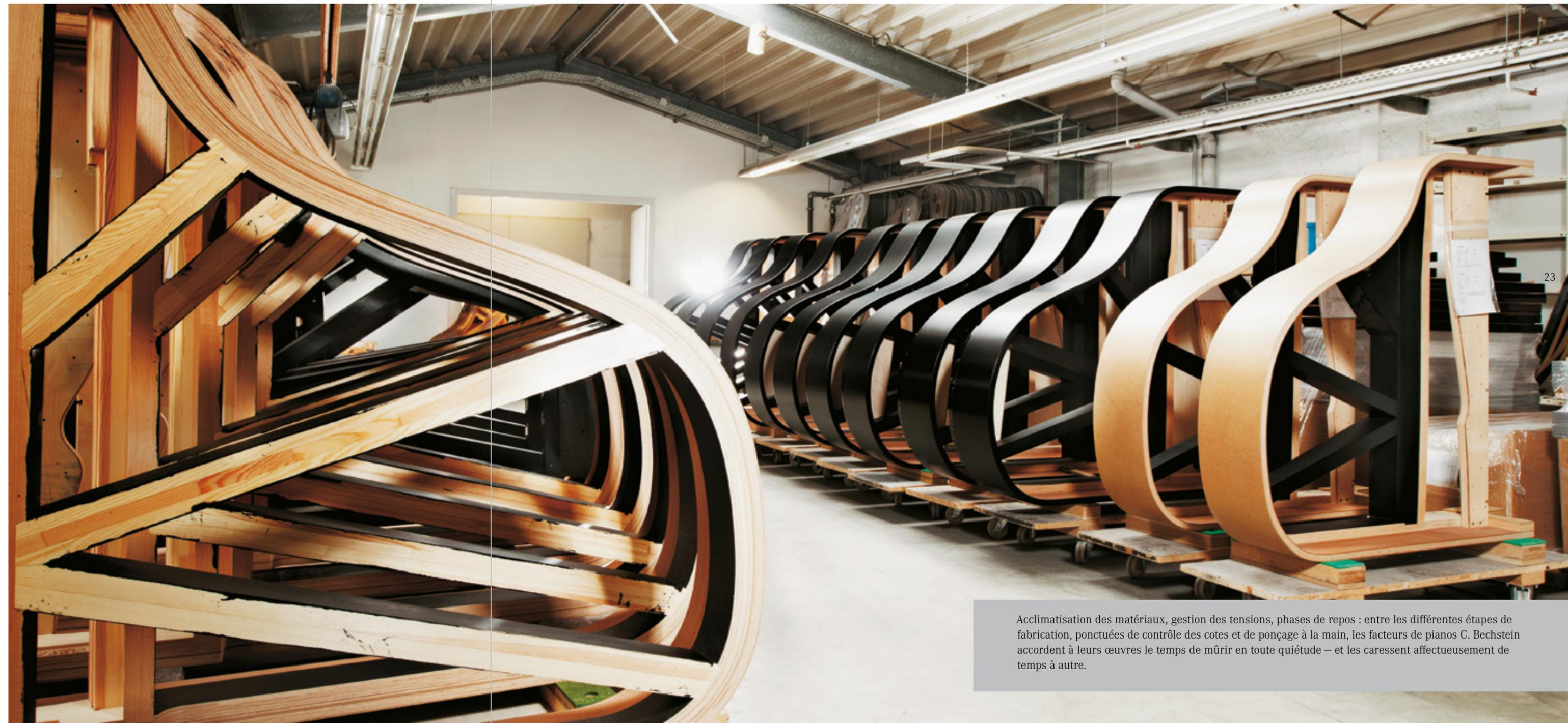
Acclimatization of materials, management of tensions, rest phases : between the different stages of production, punctuated by control of dimensions and hand sanding, the factors of C. Bechstein accord to their works the time to mature in complete quietude – and caress them affectionately from time to time.
